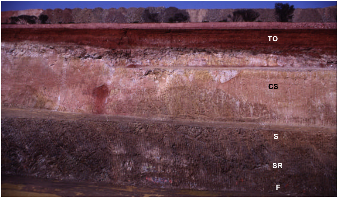
Figure 10: Regolith stratigraphy, the SW wall of the Federal open pit. Key: F – fresh rock, SR – saprock, S – saprolite, CS – clay saprolite, TO – transported overburden.
